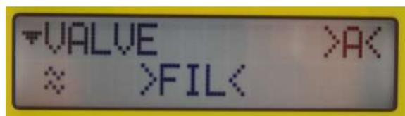
PUMP ON + VALVE in AUTOMATIC >A< (example)
